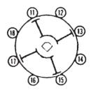
Additional Customer Decks Same As Deck 1 Except Terminal Numbers. (Deck 2: 21 to 28, Deck 3: 31 to 38, Etc)
