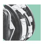
Jumpering may be done right on the switch providing a simple and neat arrangement. Silver plated brass strap jumpers are available for adjacent contacts—either between adjacent contacts on the same deck or the same terminal location on adjacent decks. Wire and lug jumpers are also available. Jumpers are already supplied assembled on the typical instrument switches, illustrated in this catalog, simplifying field wiring. All you need to do is connect the instrument leads and the line wires.
