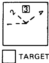
Fig. 8. Handle positions using target nameplate
